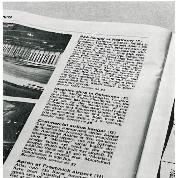
An extreme example of veiling glare is shown on the left (Fig 1a). Removal of the horizontally polarized light completely eliminates it and makes the print clearly visible (Fig 1b).
