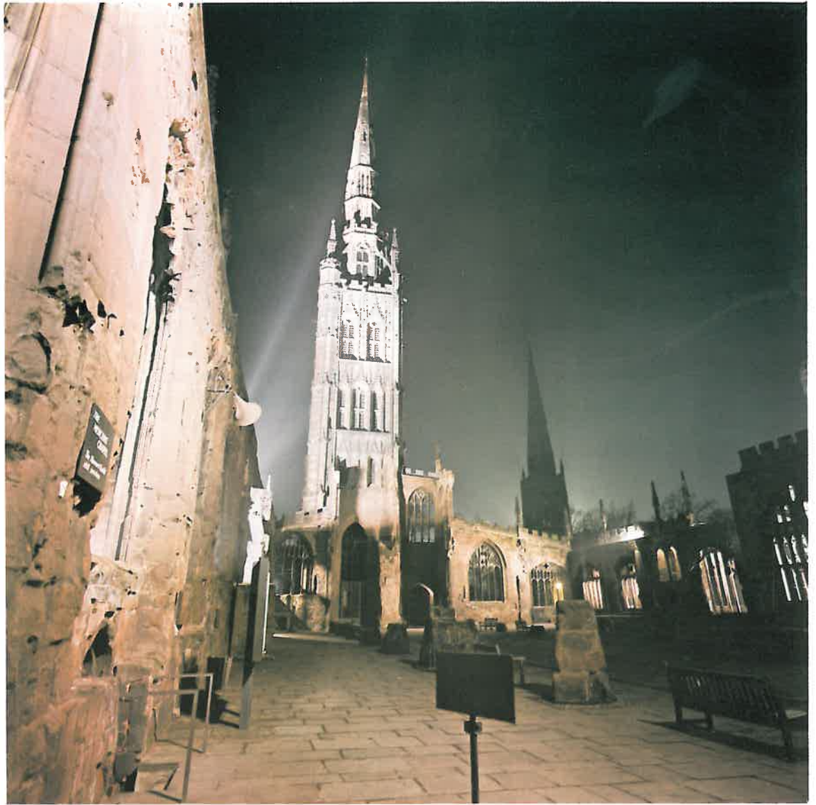
Above: Looking back from the South East corner of the ruins emphasises how the warm tones in the stone were brought out by the use of conventional tungsten filament lamps.
